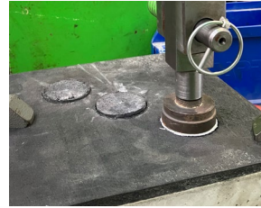
Testing tear resistance of the bonding layer ensures long-lasting adhesion to the concrete
