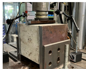
High shear resistance of the EPP tested by the Technical University of Munich
