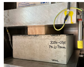
The load applied during the stackability test corresponds to the weight of 15 concrete sleepers with EPP
