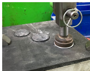
Testing tear resistance of the bonding layer ensures long-lasting adhesion to the concrete
